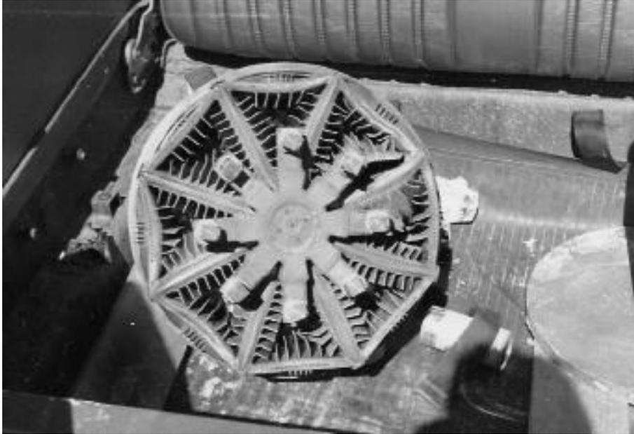
*The Blue Flame's damaged heat exchanger.*
