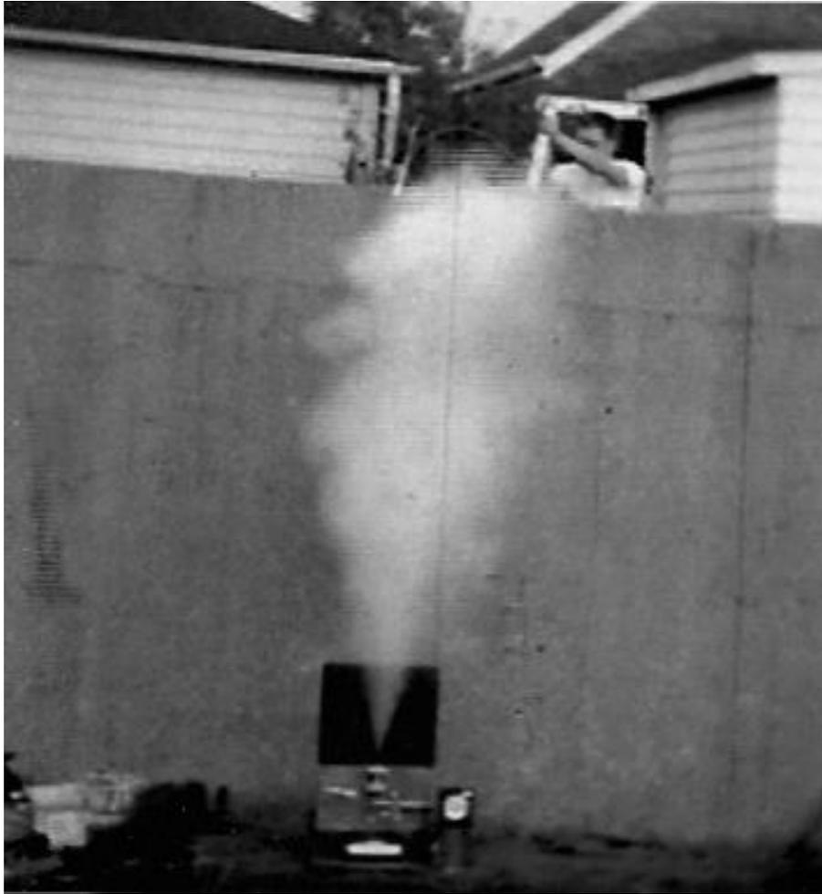
*Testing our 25 lb thrust rocket engine in the Blue Island alley*
